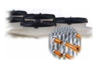
The highly efficient and compact Cross finned coil type are designed with corrugated surface aluminum fins and extended surface in inner tube. Outdoor fan with best quality fan made convenience with low noise level , saving energy and high ambient resistance temperature use until 60  $_{\circ}$  C . Axial type with external rotor motor , IP 54 motor protector and Class F insulation ( DIN EN 60 034-1 )
